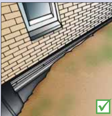
ND "Clic" Profile prevents ND 120 Drainage Composite from folding and sliding
